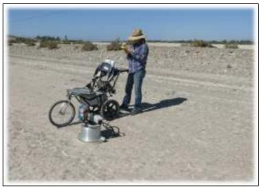
Portable In Situ Wind Erosion Lab
