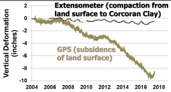
Conclusion: most of deformation is occurring below the top of the Corcoran Clay
