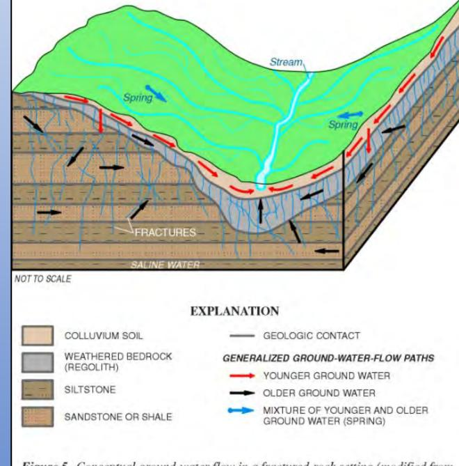
Figure 5. Conceptual ground-water flow in a fractured-rock setting (modified from Harlow and LeCain, 1991).
