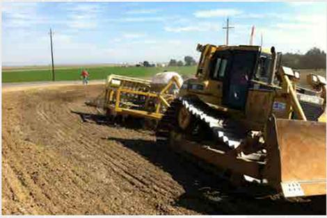
Ridger-Roller Seeder was fabricated to apply native grass seed to levee slopes.
