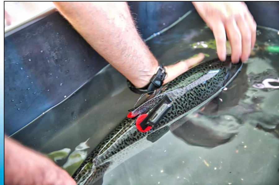
Vemco V-13 transmitter attached to salmon
