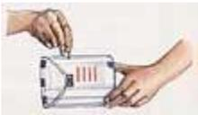
Using a ruler, measure out a scale (in millimetres) on a piece of paper. Either stick this to the side of the bottle, or use the marker pen to mark out the lines instead. Alternatively, cut the coloured tape into strips and stick them a certain distance apart (eg: 10 mm) up the side of the bottle. Make sure that whatever you use, it is waterproof!
