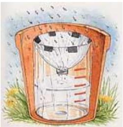
To prevent the rain gauge from blowing over, place it outside in a heavy flowerpot. Alternatively, you could dig a hole in the ground for it to stand in. Make sure the rain gauge is placed in an open area. If it is near any trees or buildings, extra water could drip into it and your measurements will not be accurate.
