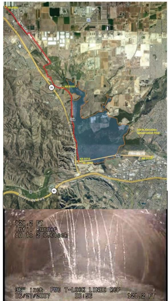
RBF also provided final design of repairs to the approximately 11 miles of 27-inch, 36-inch and 42-inch unlined RCP, including addressing a number of infiltration leaks on Reach IV-B using pressure grout injection. The project identified twelve joints with varying degrees of infiltration. Each joint was sealed followed by a video inspection of the completed work. The project also included clearing of a 10-foot wide access road along the pipeline to provide access to existing manholes.
