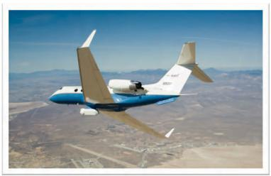
The UAVSAR L-band radar is housed in a pod flown on the NASA G-3 platform, shown here in flight over Edwards Air Force Base.
