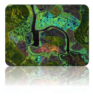
Radar remote sensing offers great potential for high resolution monitoring of ground surface changes and water extent over large areas at one time.
